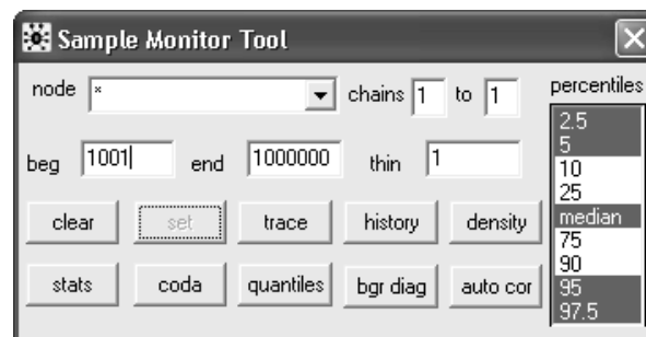
Figure B.12 How to request posterior distribution statistics for all four monitored nodes. Enter an asterisk in the node field then click stats and density.
