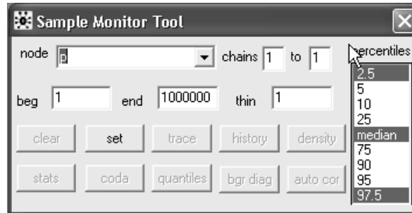
Figure B.6 The Sample Monitor Tool. Enter each node to be monitored clicking “set” after each entry
